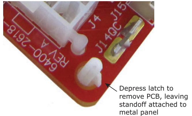
Figure 91. Remove PCB
