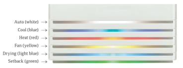
The LED bar indicates the operation status by lighting and blinking with different colors and brightness (High/Low), or by turning off. Multiple operation status indicators include blue (Cooling), light blue (Drying), yellow (Fan), white (Auto), green (Setback), red (Heating) and lime (Energy Save). Advanced settings are available for selecting desired color per mode, LED brightness (in conjunction with room brightness sensor), and temperature range indicator.
