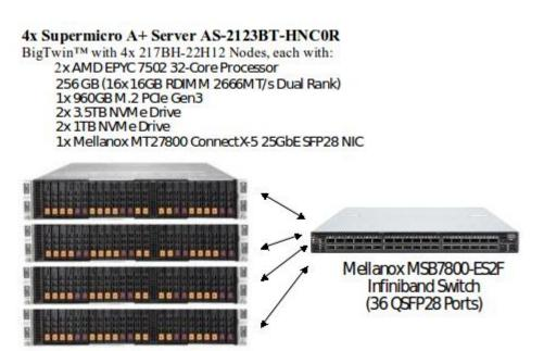
The measured configuration consisted of:
