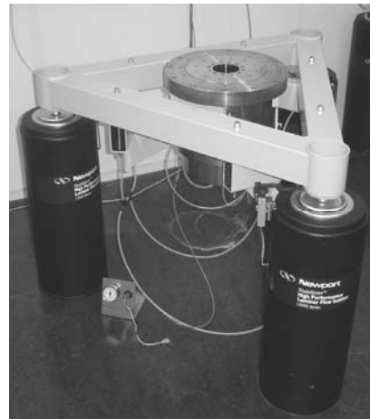
Figure 3.32: Air bearings spindle cross-section and in test setup
