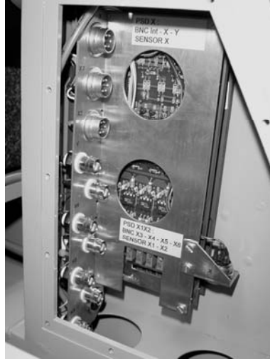
Figure 5.29: Probe electronics inside Z-stage preload frame
