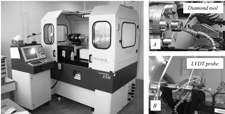
Figure A.3: The Precitech Nanoform 350 diamond turning machine at TNO, manufacturing of off-axis parts (A), and on-machine LVDT probe (B)
