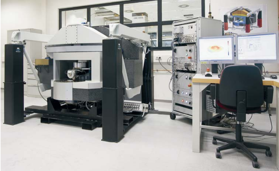
Figure 7.1: Non-contact freeform optics measurement machine prototype
