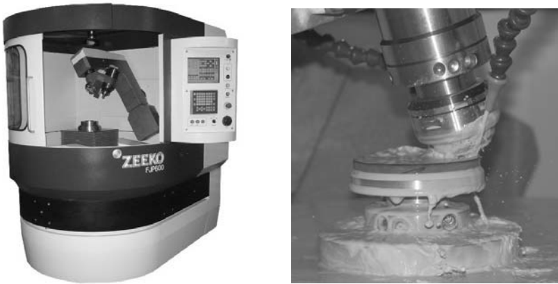
Figure A.4: Zeeko polishing robot (with FJP setup) at TNO, and classical bonnet polishing close-up
