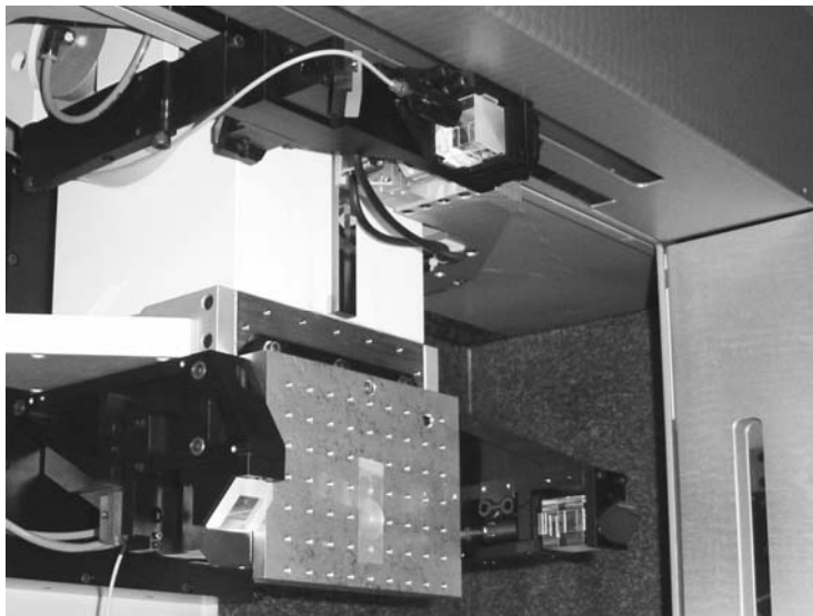
Figure 4.17: Interferometry system as assembled on the machine
