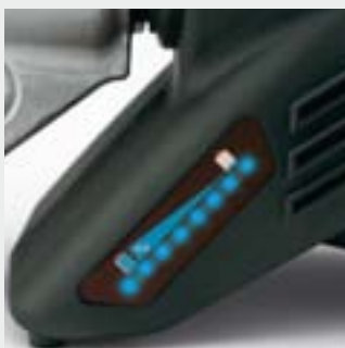
Battery condition display
