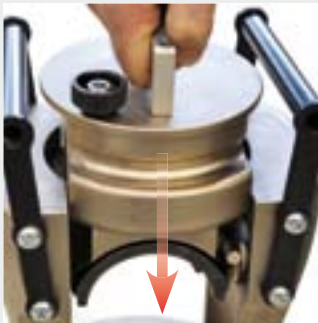
After substitution of the dies, insert the die cap into the head.
