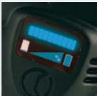
Battery condition display
