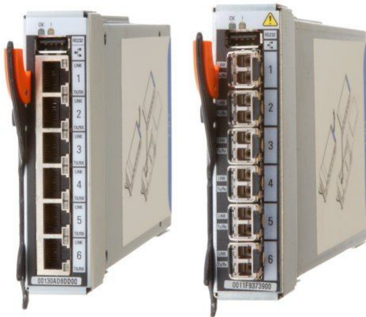
Figure 1. IBM BladeCenter Layer 2/3 Copper (left) and Fiber (right) Gigabit Ethernet Switch Modules
