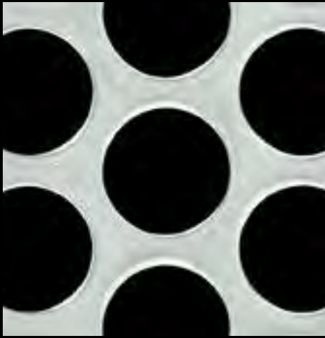
Perforated Metal, Stainless Steel Type 304, 11 Gauge, 1" Round on 1-1/4" Staggered Centers, 58% Open Area
