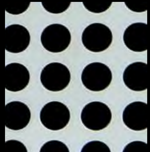
Perforated Metal, Aluminum Type 5005-H34, .125" Thick, 3" Round on 4" Straight Centers, 45% Open Area
