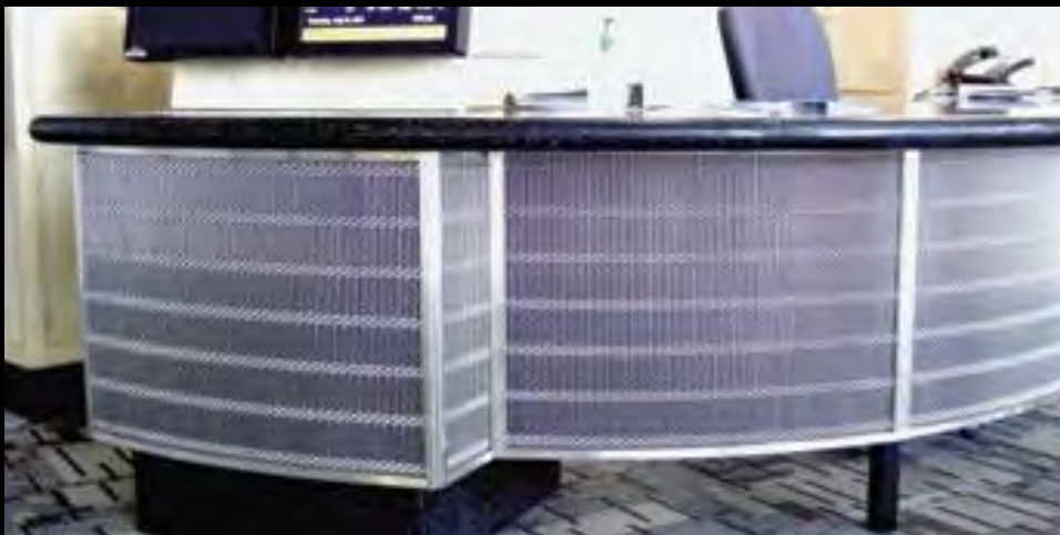
McNICHOLS® Designer Wire Mesh, AURA™ 8857, Stainless Steel Type 304, 48% Open Area, was used to transform this airport information desk into a striking display.
