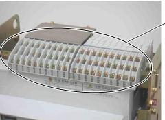
Auxiliary switch terminal screw (Control terminal screw) (Position switch terminal screw) Pan head  $M4 \times 8$ , with spring washer and terminal washer Tightening torque: 1.3 - 1.7 N⋅m
