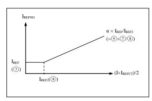
Fig. 53 Relationship between the current flowing through the ACB and the line side ground fault protection trip pickup current under "strained" conditions
