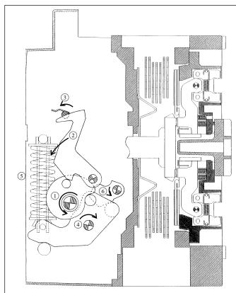
The charging handle or the charging motor provides a counterclockwise rotation to charging cam ①. This rotates closing release lever ② and closing tripper lever ③ counterclockwise and a semicircular pawl engages with closing release lever ②. And charging lever ④ rotates clockwise so that closing spring ⑤ is compressed and closing cam 5 rotates counterclockwise. At this time, each component is positioned as shown in Fig. 17
