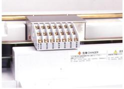
Fig. 8 Control circuit terminals
