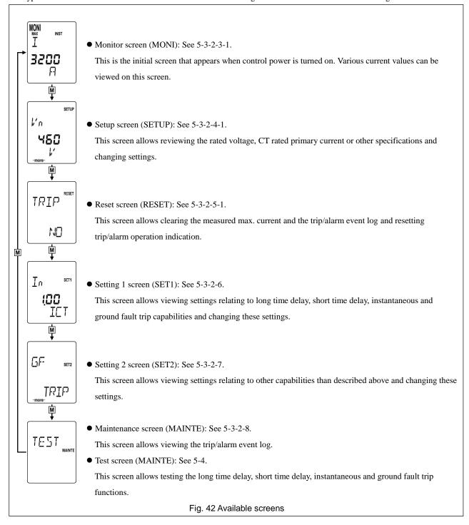
The type AGR-31B OCR has seven screens available as shown in Fig. 43 below. Press the MENU button to go to the next screen.
