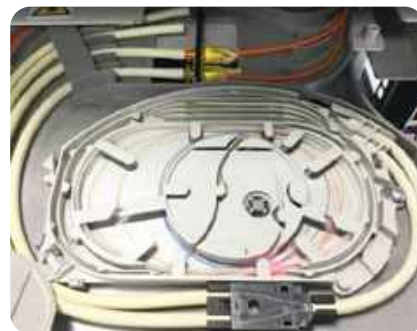
Macrobend easily visible in splice tray using 180XL
