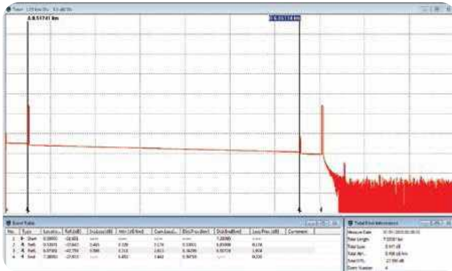
TraceViewer with expanded trace view highlighting the benefit of Launch Cables to examine Near & Far end connectors.
