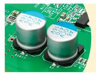
Unlike normal switch hardware design with Electrolytic capacitors (E-cap), the Zyxel Nebula Cloud Managed Switches adopt solid capacitors to get rid of drying out, bursting and leaking problems. Solid capacitors ensure Nebula switches with longer lifetime, high stability and robust operation.
