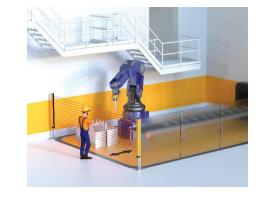
A control system that executes an active protective measure is said to carry out a **safety function** and the control system itself is called **Safety Related Control System**.
