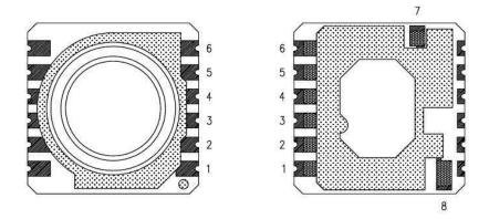
Fig. 2: Pin configuration of MS5534C
