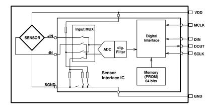
Fig. 1: Block diagram MS5534C
