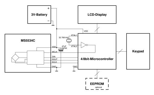
Figure 7: Demonstration of MS5534C in a mobile altimeter
