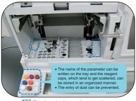
Place for storing the caps of containers for reagents, diluent and washing solution separately
