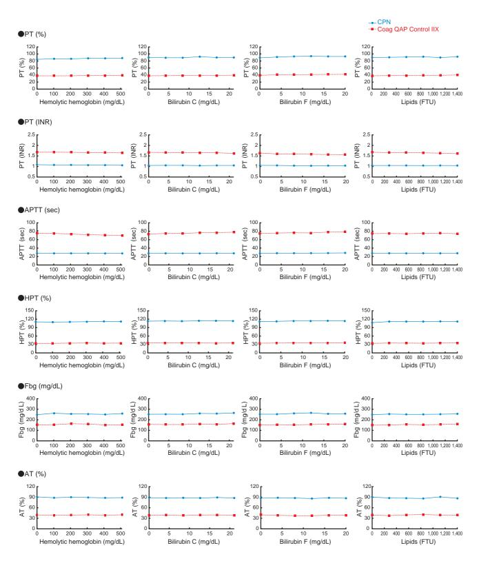
Fig. 1 Effect of interfering substances
