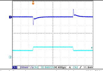
Figure 5: Output voltage response to step-change in load current (50 % -75 % -50 % of lout(max); dI/dt = 0.6 A/µs). Load cap: 15 µF tantalum cap and 1 µF ceramic cap. Ch 1: Vout, Ch 2: lout (10 A/div).
