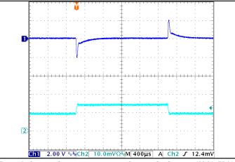
Figure 5: Output voltage response to step-change in load current (50 % -75 % -50 % of Iout(max);  $dI/dt = 0.6 A/\mu s$ ). Load cap: 1  $\mu$ F ceramic cap. Ch 1: Vout, Ch 2: Iout (1 A/div).
