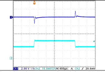
Figure 5: Output voltage response to step-change in load current (50 % -75 % -50 % of Iout(max); dI/dt = 0.6 A/µs). Load cap: 1 µF ceramic cap. Ch 1: Vout, Ch 2: Iout (1 A/div).
