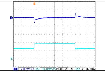
Figure 5: Output voltage response to step-change in load current (50 % -75 % -50 % of lout(max); dI/dt = 0.6 A/µs). Load cap: 15 µF tantalum cap and 1 µF ceramic cap. Ch 1: Vout, Ch 2: lout (10 A/div).
