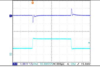
Figure 5: Output voltage response to step-change in load current (50 % -75 % -50 % of lout(max); dI/dt = 0.6 A/µs). Load cap: 15 µF tantalum cap and 1 µF ceramic cap. Ch 1: Vout, Ch 2: lout (2 A/div).
