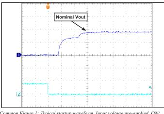
Common Figure 1: Typical startup waveform. Input voltage pre-applied, ON/ OFF Pin on Ch 2. Output voltage normalized. Timebase: 4msec/div.
