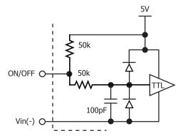
Figure B: Internal ON/OFF pin circuitry
