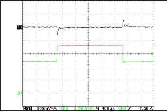
Figure 5: Output voltage response to step-change in load current (50 % -75 % -50 % of lout(max); dI/dt = 0.6 A/ $\mu$ s). Load cap: 15  $\mu$ F tantalum cap and 1  $\mu$ F ceramic cap. Ch 1: Vout, Ch 2: lout.
