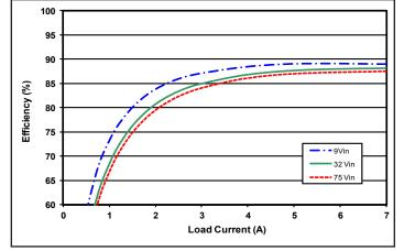
Figure 1: Efficiency at nominal output voltage vs. load current for minimum, nominal, and maximum input voltage at 25 °C.
