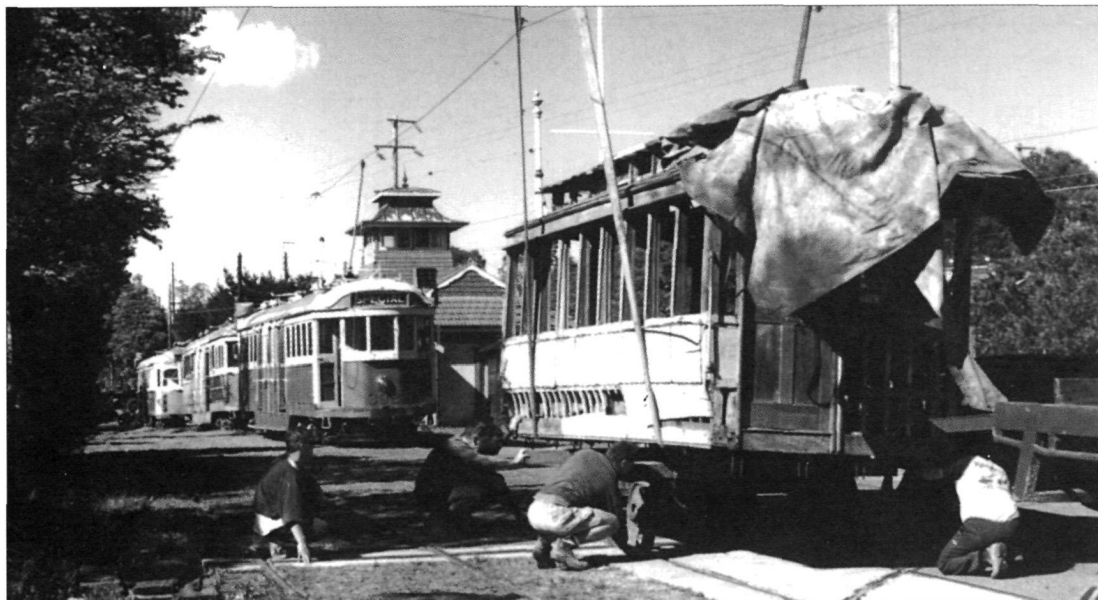
The body of C class 33 is lowered onto a trolley at Loftus on the morning of 14 October 1995.
