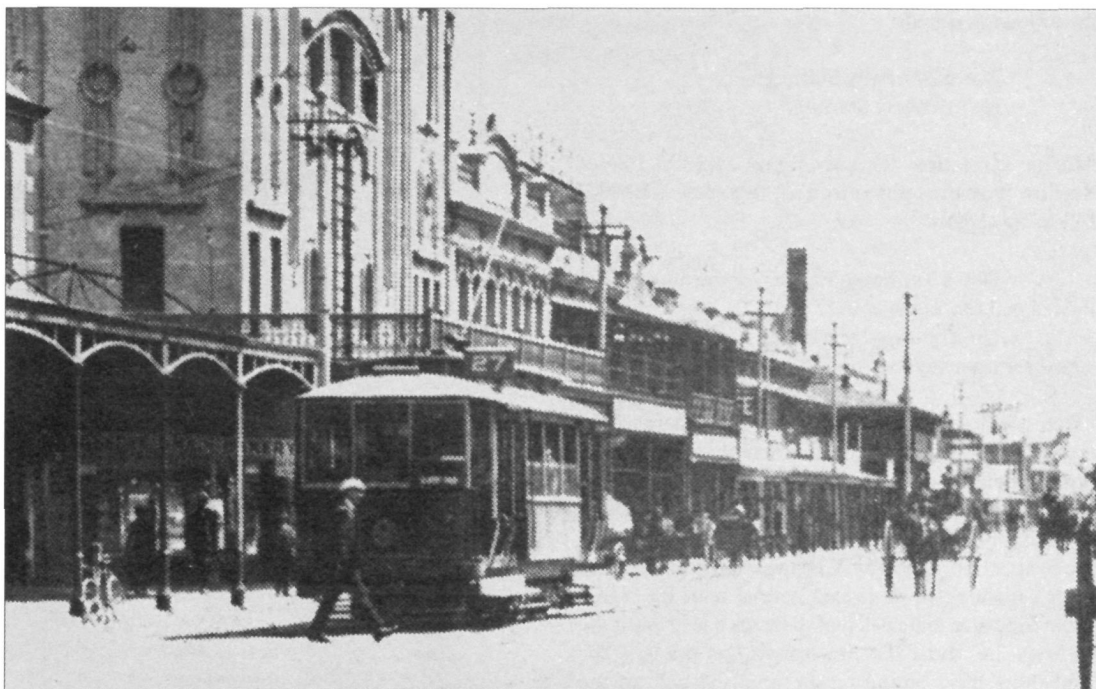
A2 "tank" tramcar No. 42 in St Vincent Street, Port Adelaide en route to Albert Park in 1922. This tram has been reconstructed to its original toastrack style by the AETM.
