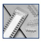
and spin-outs. Values can be read with any hematocrit tube reader. Tip-proof Identi-Tray has 24 numbered duplicate sample slots, contains enough Critoseal to seal several hundred tubes.
