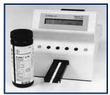
reagent strip in 1 minute vs 2 minute visual reading. Flags abnormal results. Computer interfaceable.
