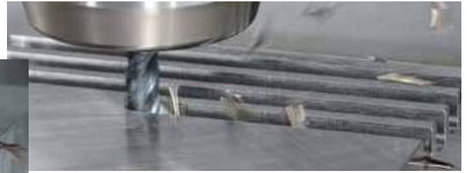
Large rake angle and unique flute design improve sharpness and excellent chip evacuation.
