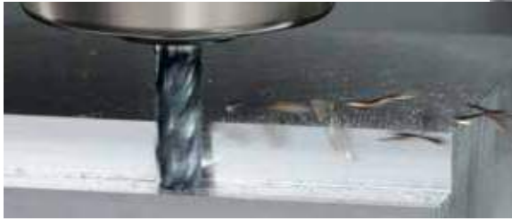
Large rake angle and unique flute design improve sharpness and excellent chip evacuation.
