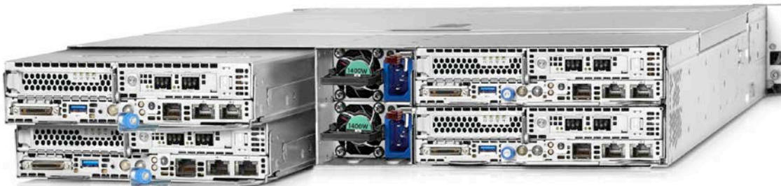
Chassis, back view with 4 nodes
