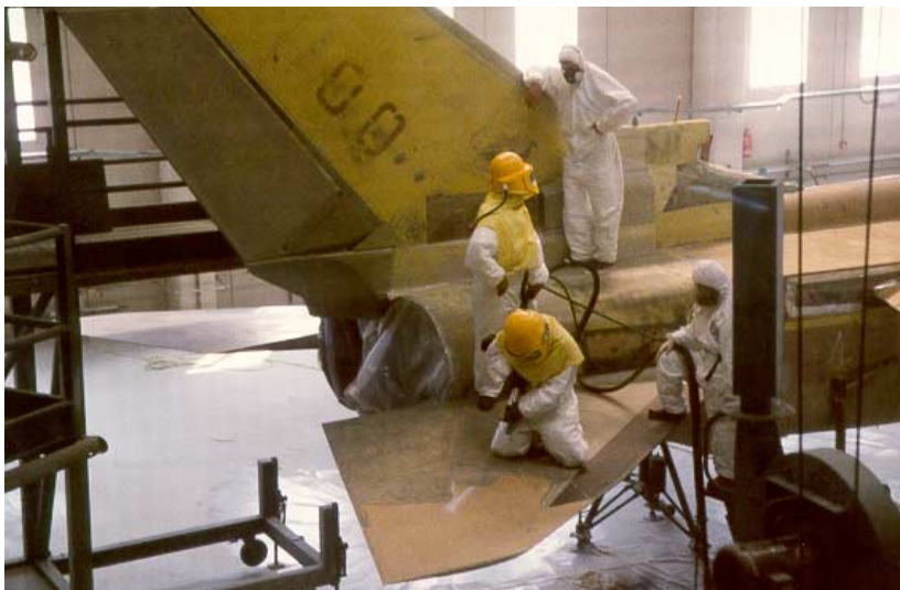
Fig. 1 – IAF Tornado stripped by means of Plastic Media
