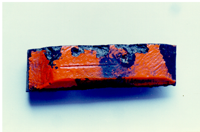
Fig. 7 – Pitting Corrosion on MB-326 Balance Tabs
