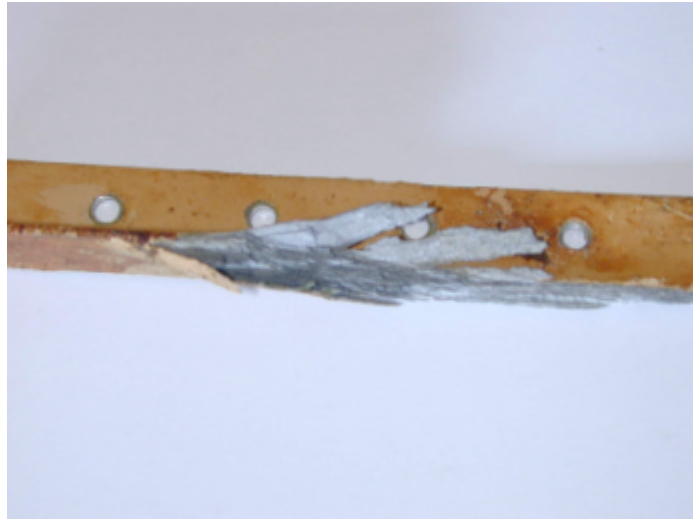
Fig. 4 – Exfoliation on a Breguet Atlantic Br.1150 AA2024 spar
