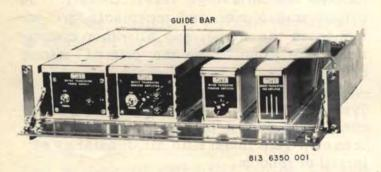
Fig. 3 - Shelf Assembly With Guide Bar
