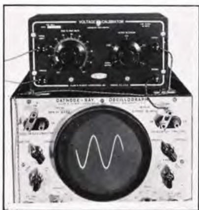
Figure 1. Signal voltage is passed through the Voltage Calibrator to the Vertical Input of the Cathode-ray Oscillograph. The signal voltage appears on the screen.
