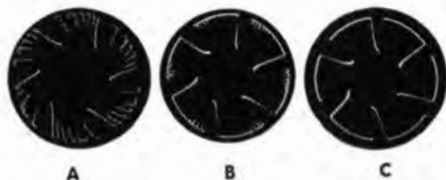
Figure 1. Oscillograms taken from the Type 275-A in adjusting the spring tension on the distributor contact points in a 6-cylinder engine. Oscillogram A indicates excessive bouncing of the contact points, B indicates a moderate degree of bounce, and C corresponds to proper adjustment of the tension
