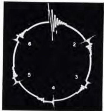
Figure 5. A typical oscillogram resulting from the set-up shown in Figure 4. Each of the six oscillations on the circular time-base is a plot of the voltage across the coil primary at the time when the spark plugs fire. Interpretation of the oscillogram shows that plugs 2, 3, 5, and 6 are firing normally, while plug 1 is open and 4 is shorted
