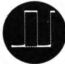
Response of an amplifier to a square-wave signal
