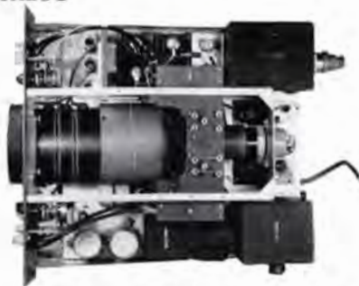
Figure 5. Top view of the Type 281 with cabinet removed. Note accessibility of deflection plate terminals for direct connections
