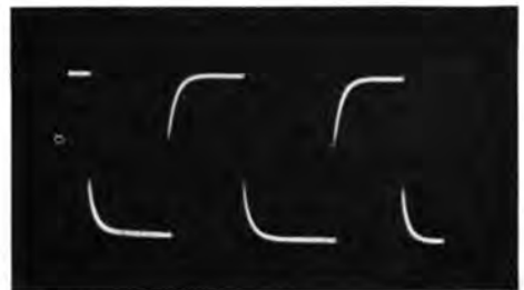
Figure 4. Oscillograms illustrating the effect of a high-impedance gain control upon amplifier band-width. They were made with maximum gain (left) and with reduced gain (right)
