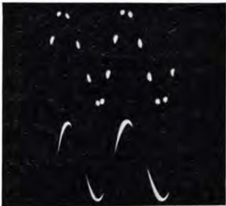
Figure 6. Oscilloscope showing intensity modulation by signals of different frequencies. At the top, a 60-cycle signal is intensity-modulated at 120 cycles per second. At the bottom, the same 60-cycle signal is modulated at 480 cycles per second
