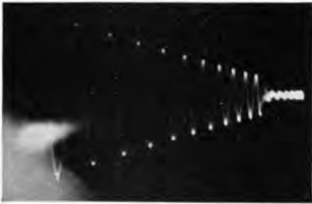
Figure 1. Unretouched oscillogram of a high-speed transient photographed from the Type 281 operated with an accelerating potential of 8,000 volts. Photograph made with a Du Mont Type 271-A Oscillograph-record Camera having a lens speed of f/3.5 . Writing speed in the first cycle of the transient is 13 inches per microsecond; in the 10th cycle 3.5 inches per microsecond
