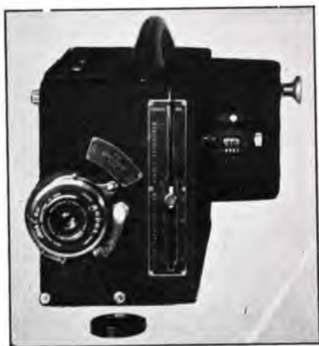
Figure 6. Front view of Type 314 Camera showing the lens, the manually operated lever for film advance after single exposures, the footage indicator which shows the exposed film length, and the push-pull knob on the side to actuate the clutch.
