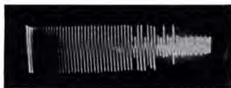
Figure 4. Single exposure photographic recording of the starting-current characteristic of a synchronous motor.
