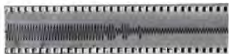
Figure 3. Continuous motion recording of starting current in a synchronous motor under load. Current is switched from starter winding as motor builds up torque. Timing markers are unnecessary since each cycle represents 1/60 second. Motion of film provides time base.
