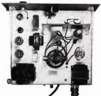
Figure 1. Top View of Chassis. The simplicity of this high voltage power supply and its comparatively light weight both result from the use of a rectified, high-voltage, radio-frequency signal to supply the output power.
