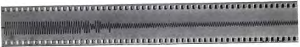
Figure 5. Moving-film recording of the same starting-current characteristic as is shown in Figure 4.
