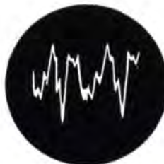
G-392 cycles per second as produced by a single reed of an accordion
