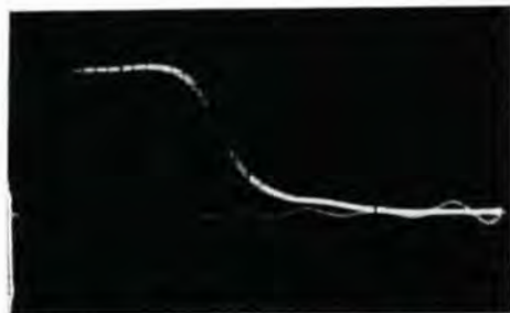
Figure 5. The leading edge of a horizontal synchronizing pulse as plotted on the 1 microsecond sweep of the Type 280. Expansion of the pulse amplitude is accomplished by using the positive-peak-clipping circuit
