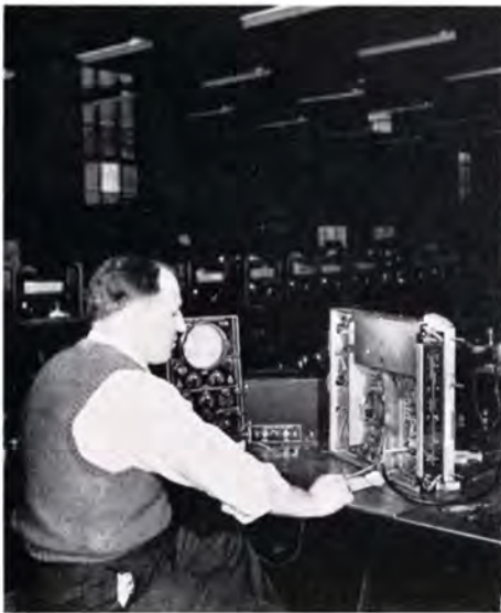
Figure 3. The Type 208-B Cathode-ray Oscillograph in use in the testing of television circuits at our own factory
