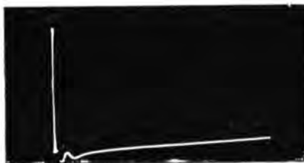
Figure 2. A sharp pulse displayed on the 5 microsecond sweep with no delay in vertical amplifier
