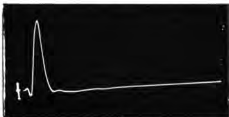
Figure 3. Same as Figure 2, with delay network inserted in vertical amplifier. Note that entire pulse is now visible, whereas without the delay network it had occurred before the sweep could get started
