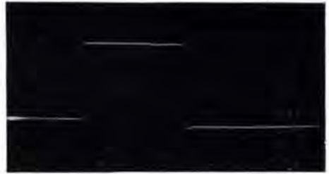
Figure 2. Oscillogram taken from the Type 256-D showing a square pulse of 1 microsecond duration after it has passed through the vertical amplifier. Note the reproduction of the extremely fast rise and fall of the pulse
