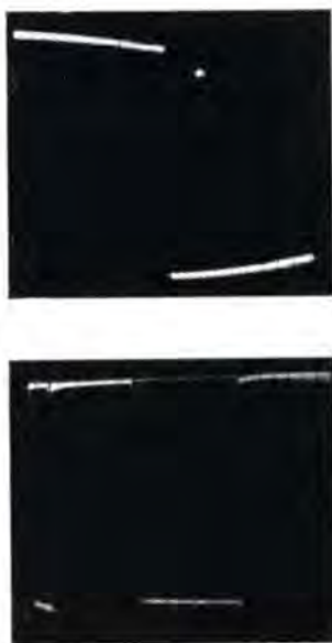
Figure 2. Response of the vertical amplifier of the Type 224-A to square-wave signals. Top oscillogram, 50 cycles per second; bottom oscillogram, 100,000 cycles per second
