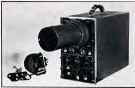
Figure 2. Convenient Disassembly. For the adjustment of shutter speeds, lens speeds, and for reloading, the camera may be simply removed from the light hood to which it clamps securely with a bayonet lock and spring detent. The camera body, exclusive of the mounting clamp and hood, may be removed from the oscillograph to leave the hood to serve as a convenient light shield.
