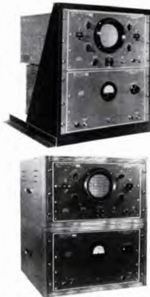
Figure 3. The Du Mont Type 281 and Type 286 are designed so that they may be used together or as separate instruments. When used together, they may be mounted in a standard relay-rack (Fig. 3A) or fastened together in their cabinets (Fig. 3B)
