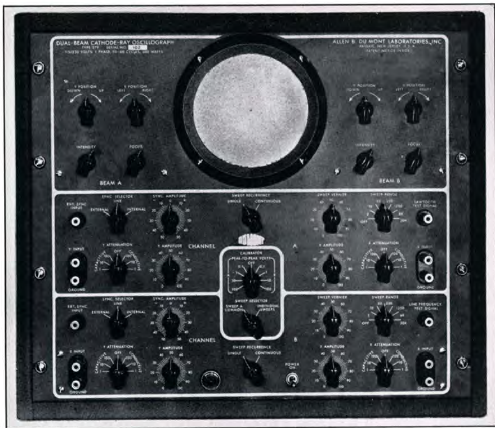
Figure 2. Front panel of the Type 279. Some idea of the instrument's versatility may be gathered by studying the number of combinations and selections which may be made. All controls are grouped and located to provide for simple operation
