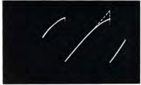
Figure 7. Oscillogram of a non-linear sawtooth voltage (solid line) showing comparison with a perfectly linear sawtooth (dotted line)
