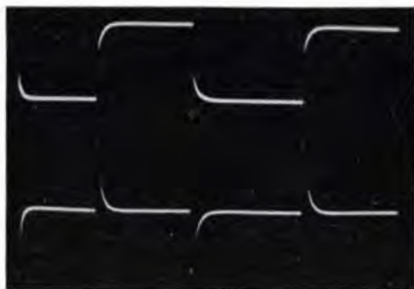
Figure 4. Oscilloscope showing a square-wave signal (top) and the resultant waveform after differentiation by an RC network (bottom). Both signals are plotted on a common sweep
