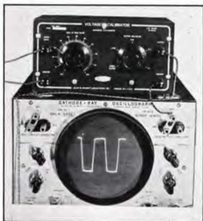
Figure 2. Same as Figure 1 except that the OUTPUT MULTIPLIER switch has been turned to the X.1 Position resulting in the calibration voltage appearing on the screen.
