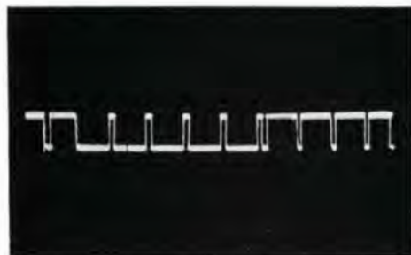
Figure 3. A vertical synchronizing pulse showing the horizontal equalizing pulses
