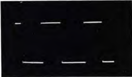
Figure 4. Oscillograms illustrating the effect of a high-impedance gain control upon amplifier band-width. They were made with maximum gain (left) and with reduced gain (right)
