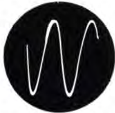
Sine wave produced by a tuning fork
