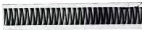
Figure 8. Continuous-motion recording of a 60-cycle sine wave signal from a P1 cathode-ray tube screen. The blurred effect is caused by the persistence of the screen material.
