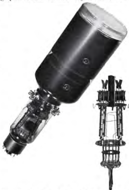
Figure 1. The Du Mont Type 5SP Dual-Beam Cathode-ray Tube showing the structure of its electron guns. The two guns are physically separate and are shielded to prevent interaction between the deflection plates associated with each
