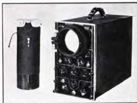
Figure 1. Clamping Ring. The body of the Type 271-A Camera passes through the clamping ring to bear against the face of the cathode-ray tube. No adjustment of focus is necessary. The rubber edge provided on the body of the camera prevents the possibility of scratching or otherwise damaging the face of the cathode-ray tube.
