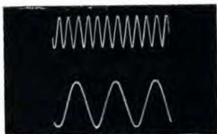
Figure 2. By adjustment of the balance control on the Type 185-A Electronic Switch, two patterns on the screen of the cathode-ray tube may be displaced with respect to each other to facilitate separate, detailed study of each
