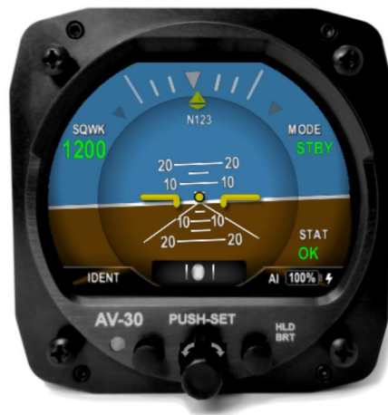
Figure 26 - Reversionary Attitude Indicator
