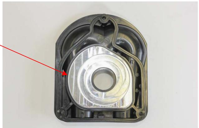
5. Insert the upper pump base with counter plate in the opening of the spiral housing until it stops. Screw the upper pump base with the spiral housing using the three cylindrical screws with hexagon socket (M8). To fasten the screws, medium-strength screw locking (Loctite) is to be used. Please refer to Table 6.4.1 for the correct screw tightening torque.
