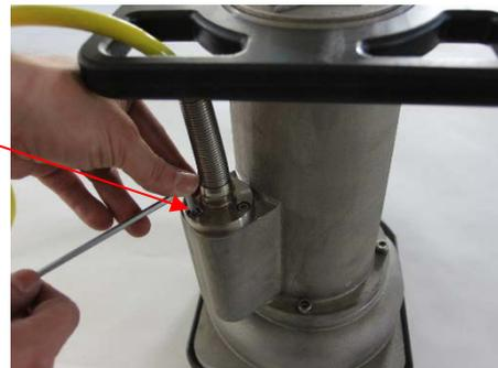
2. Unplug the cable screw connection including plug and coupling from the housing. Open the connection cable plug and unplug the cable from the coupling.
