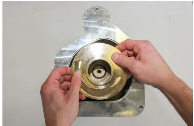
6. Remove the blockage cause from the spiral housing and the impeller.
