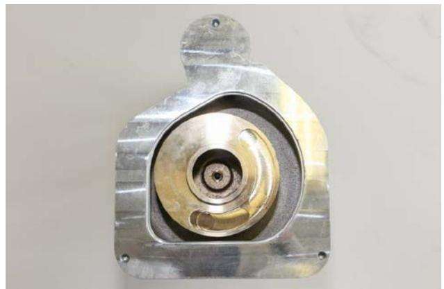
3. Screw the impeller with the motor shaft using the cylindrical screw with hexagon sockets (M8). To fasten the screws, medium-strength screw locking (Loctite) is to be used. Please refer to Table 6.4.1 for the correct screw tightening torque.
