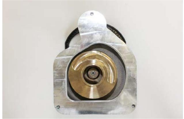
4. Remove the cylindrical screw with hexagon sockets (M8) from the impeller. Hold in place by using a mounting iron placed in the impeller opening. Open the screw anti-clockwise with a suitable spanner.
