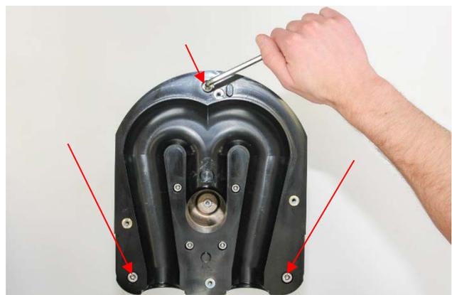
3. Remove the upper pump base from the spiral housing.
