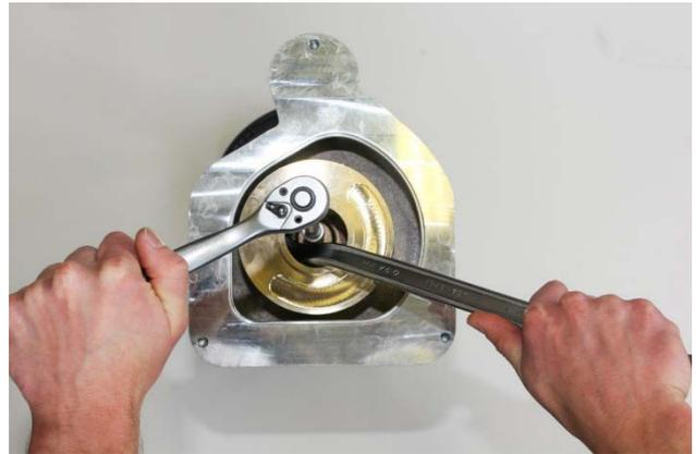
5. Remove the impeller from the shaft. if it is difficult to remove, take a conventional M10 screw and screw this on to the impeller (the thread is inside the impeller) until resistance can be felt. Continuing screwing to press the impeller away from the shaft. Then clean the polygon connection and check for damage.
