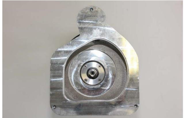
2. Evenly place the impeller on the motor shaft and push it down until it stops.
