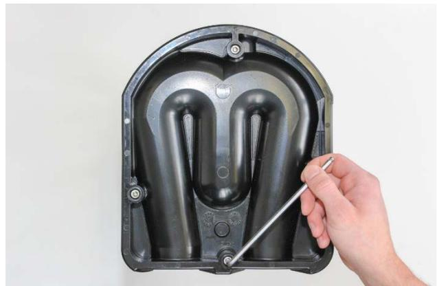
2. Remove the three cylindrical screws with hexagon socket (M8) which connect the upper pump base with the spiral housing.
