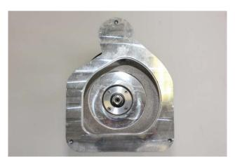
2. Evenly place the impeller on the motor shaft and push it down until it stops.
