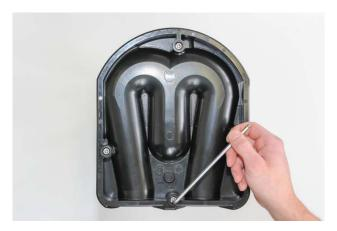
Remove the three cylindrical screws with hexagon socket (M8) which connect the upper pump base with the spiral housing.
