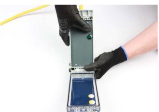
Close the housing again and then reinsert the power plug. If the motor protection switch triggers again, see points 7 and 6.3.
