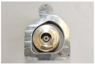
3. Screw the impeller with the motor shaft using the cylindrical screw with hexagon sockets (M8). To fasten the screws, medium-strength screw locking (Loctite) is to be used. Please refer to Table 6.4.1 for the correct screw tightening torque.
