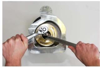
5. Remove the impeller from the shaft. if it is difficult to remove, take a conventional M10 screw and screw this on to the impeller (the thread is inside the impeller) until resistance can be felt. Continuing screwing to press the impeller away from the shaft. Then clean the polygon connection and check for damage.
