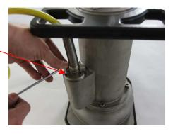
Unplug the cable screw connection including plug and coupling from the housing. Open the connection cable plug and unplug the cable from the coupling.
