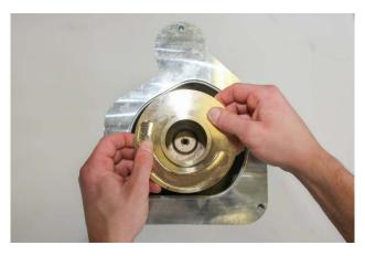
6. Remove the blockage cause from the spiral housing and the impeller.
