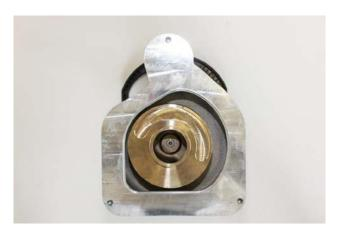
4. Remove the cylindrical screw with hexagon sockets (M8) from the impeller. Hold in place by using a mounting iron placed in the impeller opening. Open the screw anti-clockwise with a suitable spanner.
