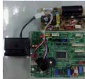
Connection of terminal block and Main PBA
