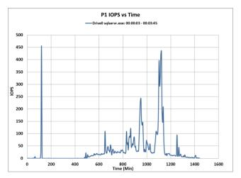
Figure 29 - Self-Test IOPS v Time. Cumulative IOPS while application runs on target server during an IO Capture
