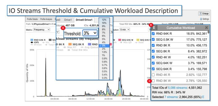
Figure 18 – Filter IO Stream Maps by IO Stream Threshold & Workload Descriptions
