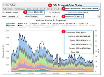
Figure 21 – 5 min Steps. Coarse grain resolution allows viewing of multiple/aggregate drive, long duration captures
