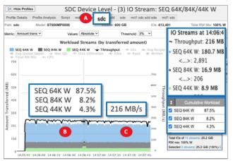
Figure 16 – IO Stream Map RAID md1. IO Stream Map showing SEQ 1204K Workload applied to RAID md1
