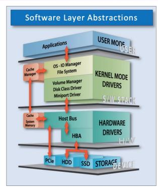
Figure 1 - SW/HW Stack. IO Streams merge, append, coalesce and split as they traverse the SW/HW Stack
