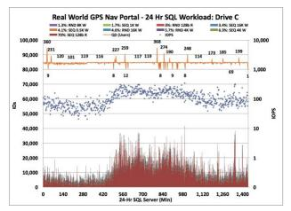
Figure 12 - GPS Nav Portal: Boot DriveC. 67:33 RW; 70% SEQ 128b R; Median QD 8, Max QD 368
