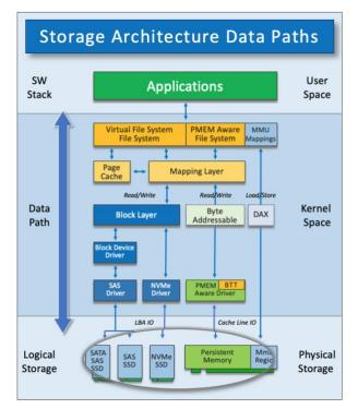
Figure 2 - Data Paths. Data Paths impact IO Streams as they are exposed to each layer of abstraction
