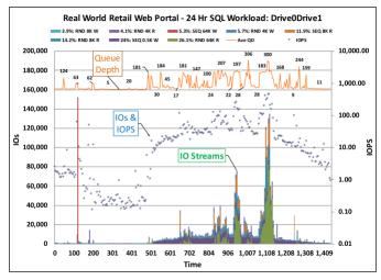
Figure 3 - Real World Workloads. Constantly changing combinations of IO Streams and Queue Depths
