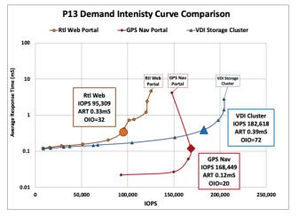
Figure 32 – DI OS Curve: GPS Nav Portal. Max IOPS shows the optimal "knee" before performance saturation
