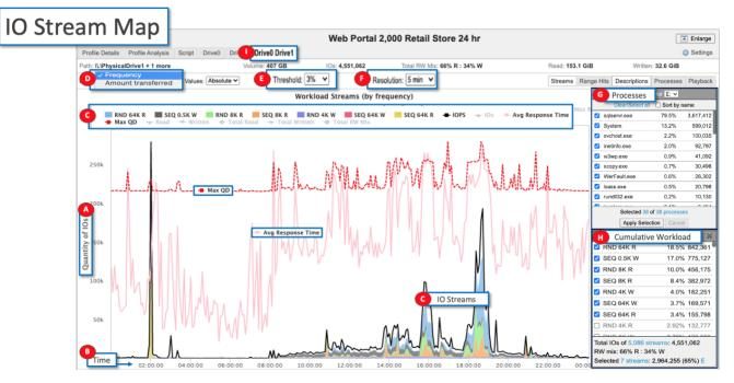
Figure 7 - IO Stream Map: Quantity of IOs v Time
