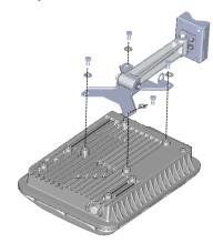
2 Use four 0.5-inch x 0.250-28 hex bolts with split lock and flat washer sets to mount the AP bracket to the AP. Tighten the bolts to 2.5-3.0 N.m or 22-27 in-lbs.
