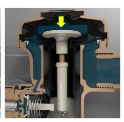
Upper chamber repressurizes through the bypass, causing diaphragm to re-seat and ending flush
