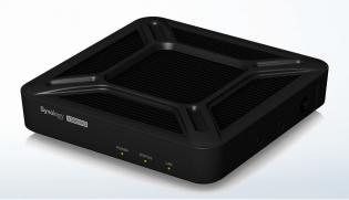
Synology VisualStation VS960HD is a compact, durable, and high-performance external display device built for Synology Surveillance Station 8 and onward<sup>1</sup>. It comes with dual HDMI outputs supporting 4K and 1080p respectively, and supports 96 IP camera streams at 720p/10FPS. Synology VS960HD is backed by Synology's 3-year limited warranty.
