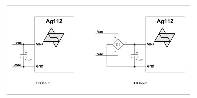
Figure 4: Input Connections – DC or AC Input
