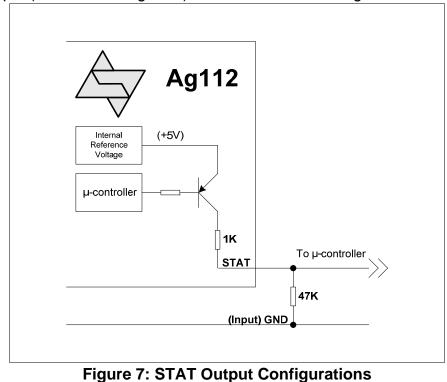
Note: Figure 7 shows a 47K pull down resistor, this is required to ensure that the open collector output switches correctly (but this is not a critical value), the STAT output can source ~5mA.
