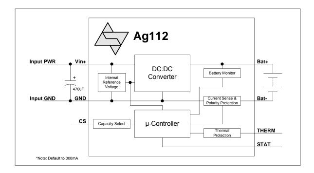
Figure 1: Block Diagram with External Components
