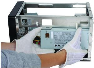
• Place the power supply in position. Secure from the back with three Phillips head screws.
