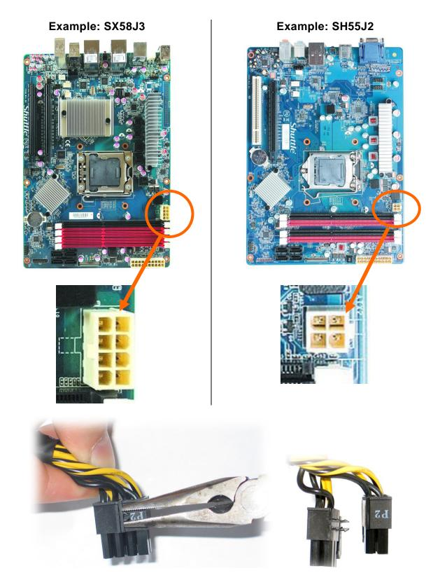
The ATX12V plug of the power supply consists of two 4-pin plugs, which can be combined to one single 8-pin plug. They can easily be separated again by using long-nosed pliers (as shown in the photo).
