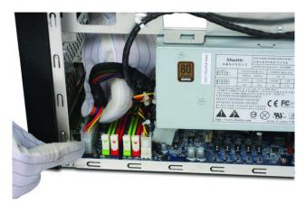
3 Attach the 20-pin ATX and 2x2-pin (or 1x4-pin) power supply plugs to the mainboard.
