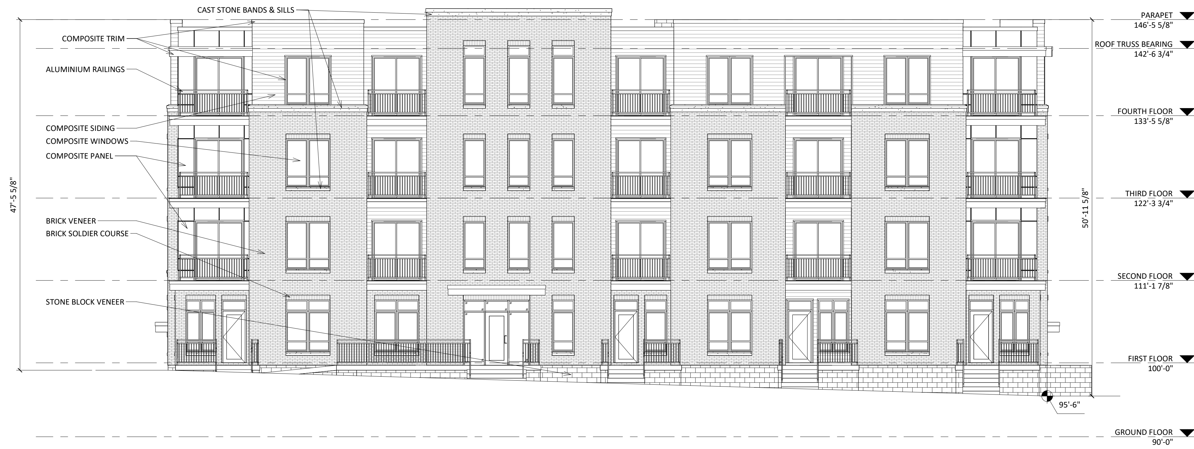
1 ELEVATION - NORTH A-2.1 1/8" = 1'-0"
