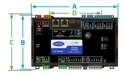
QR code on label to provide technician with access to MAC address, serial number and technical documentation
