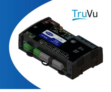
The TruVu™ Universal Controller is ideal for HVAC equipment control, advanced air quality control and most zone-level applications. The TV-UC683T features dual Ethernet ports with built-in fail-safe that supports direct connection or daisy chain topologies using BACnet/IP and 17 points of onboard control. Designed to operate in a wide range of environmental conditions, it is well suited for mechanical rooms, equipment boxes, or almost any other weather-tight location.
