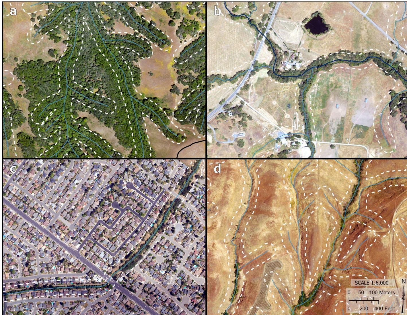
Figure 2. Aerial imagery (U.S. Geological Survey, 2022) showing examples of the riparian zone (dashed white lines) from various locations across the watershed. The riparian zone is 100 ft wide on either side of mapped streams (blue lines; SFEI-ASC, 2017). Images are A) forested headwaters of San Antonio Creek, B) the main stem San Antonio Creek, indicated by the darker blue streamline, C) East Washington Creek in the City of Petaluma, and D) gullied streams dominated by grassland vegetation in the southeast part of the watershed.
