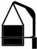
Vertical Mast (70% of Operating Load, not to exceed 6,000 pounds)
