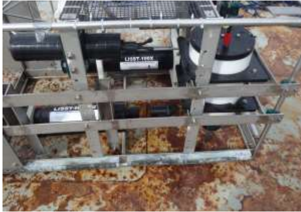
Figure 2: Illustration of the profiling frame equipped with the LISST100X, LISST HOLO2 and PCAM (left), typical profile showing the measurement strategy
