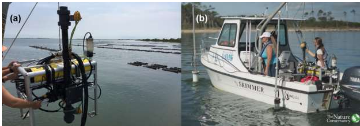
Figure 1. (a) Profiler cruise instrumentation deployed on a stationary frame, and (b) Dataflow cruise instrumentation mounted to the vessel while underway.
