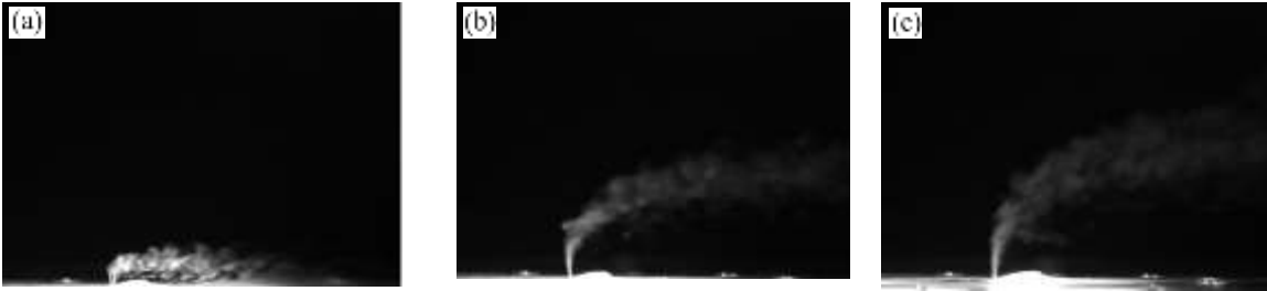
Fig. 3 Snapshots of resuspension events for a flume mean velocity u_m = 7.8 \text{ cm s}^{-1} , particle size d_{50} = 34.2 \mu\text{m} and injection flow rates of q_{sp} = (a) 6 \text{ ml min}^{-1} ; (b) 20 \text{ ml min}^{-1} ; and (c) 45 \text{ ml min}^{-1} .
