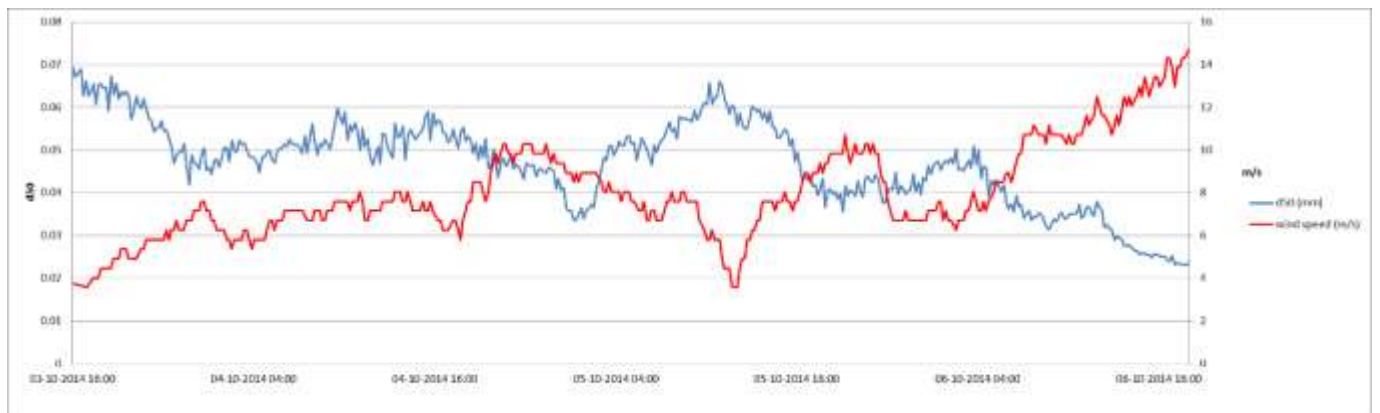
Figure 4 Grain size variation (blue curve) and wind speed variation (red curve) at position NS04a. At this site, the median grain size is inversely correlated to the wind speed. The wave energy destroys the fragile flocs resulting in a decreasing size during rough periods. The flocs reform quickly as the wind speed decrease.
