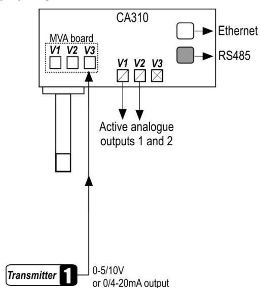
When a channel of the MVA board is enabled, the corresponding channel in output est disabled (e.g: channel n°3 of the MVA board enabled, channel n°3 in output disabled).
