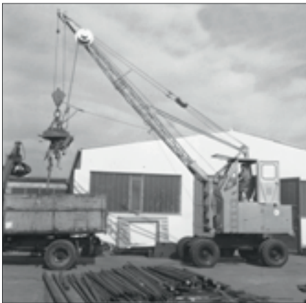
1962: rope-driven S833 with elevated operator cab
