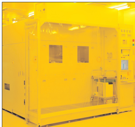
Ion implantation equipment used in SiC power semiconductor processing.
