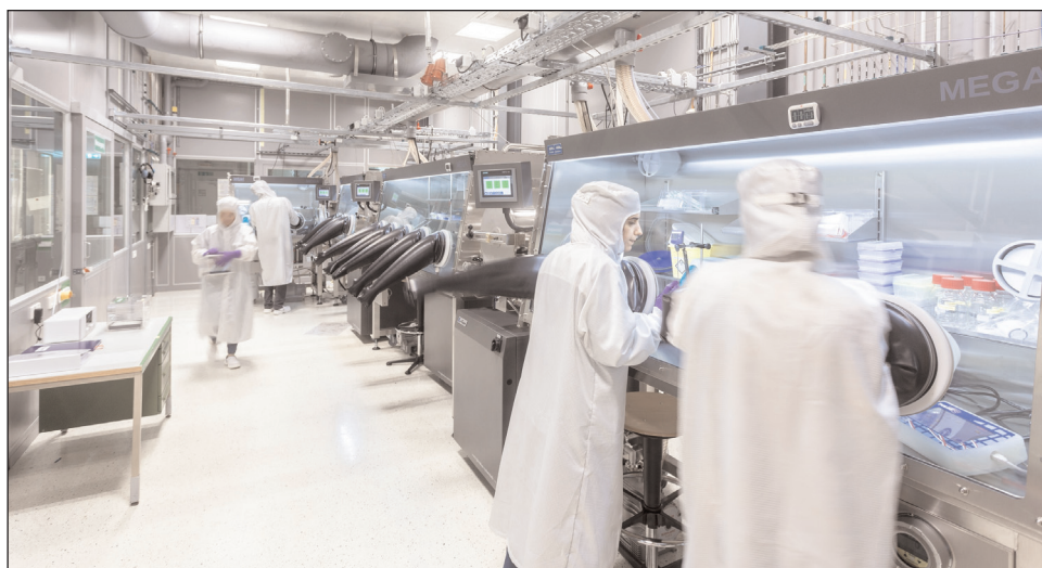
Processing perovskite–silicon tandem solar cells at Fraunhofer ISE. The lab infrastructure comprises evaporation chambers for perovskite absorbers, selective contacts and metals, and the atomic layer deposition of metal
