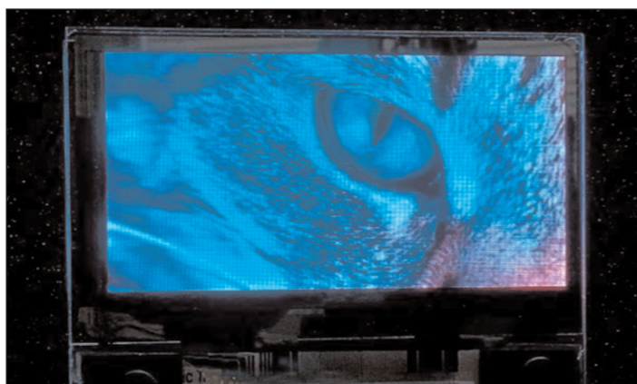
X-Celeprint's 2000cd/m 2 micro-LED display, using RPCVD p-GaN, showing good colour uniformity quantum efficiency and forward voltage.
