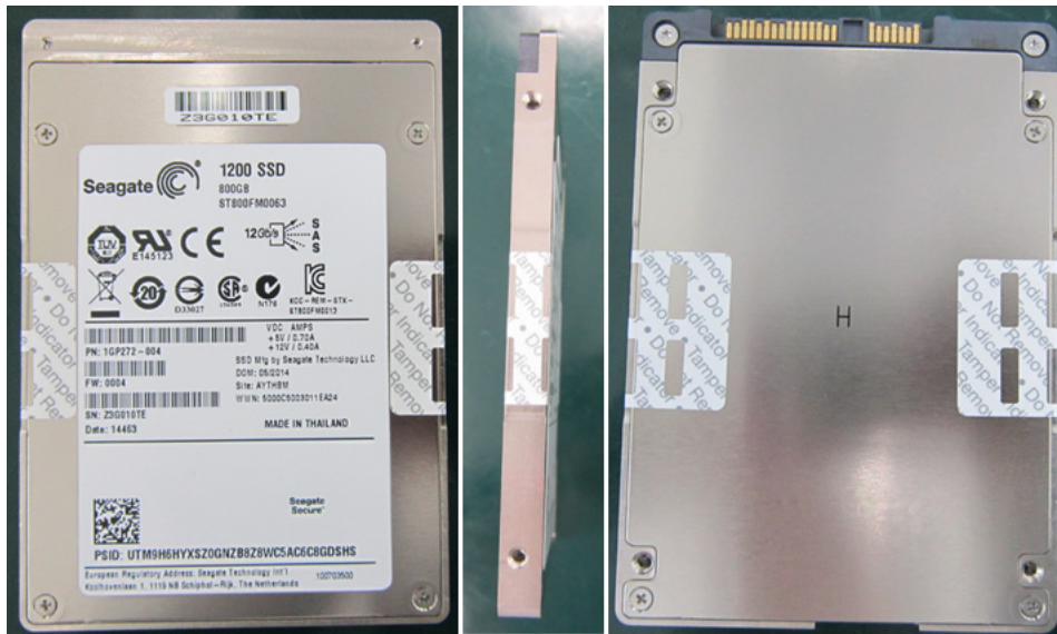
Figure 21. Example of FIPS tamper evidence labels.
