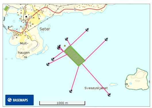
**Figure 14.** Illustration of the anchoring array of a Norwegian salmon farm (selected at random). Image copied from the Directorate of Fisheries' mapped database (<a href="https://kart.fiskeridir.no/">https://kart.fiskeridir.no/</a>)
