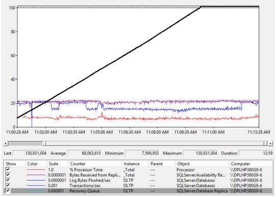
*Figure 11. Permon graphic highlighting the growth of the secondary recovery queue when the AG log transport rate exceeds the rate of the AG log redo.*
