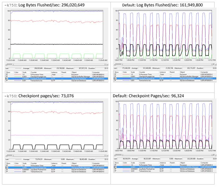
Figure 7. These perfmon metrics graphically demonstrate the benefits of leveraging the -k startup trace flag to throttle checkpoint pages at a user-defined value.
