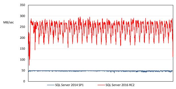
*Figure 9. This test reinforces the enhanced network log transport performance for SQL Server 2016 vs. SQL Server 2014.*
