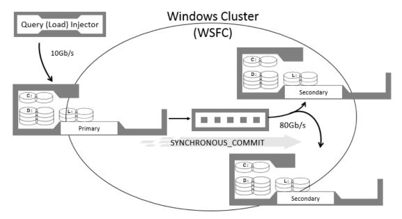
Figure 2. Architecture diagram. The workload is consumed by the primary replica.
