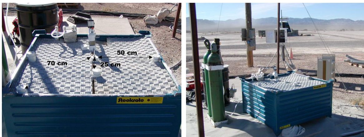
Figure 22. Sandbox Test. Left: Placement of tubes for contaminant (center tube) and sensors. Right: Sandbox with data-logging station in background.
