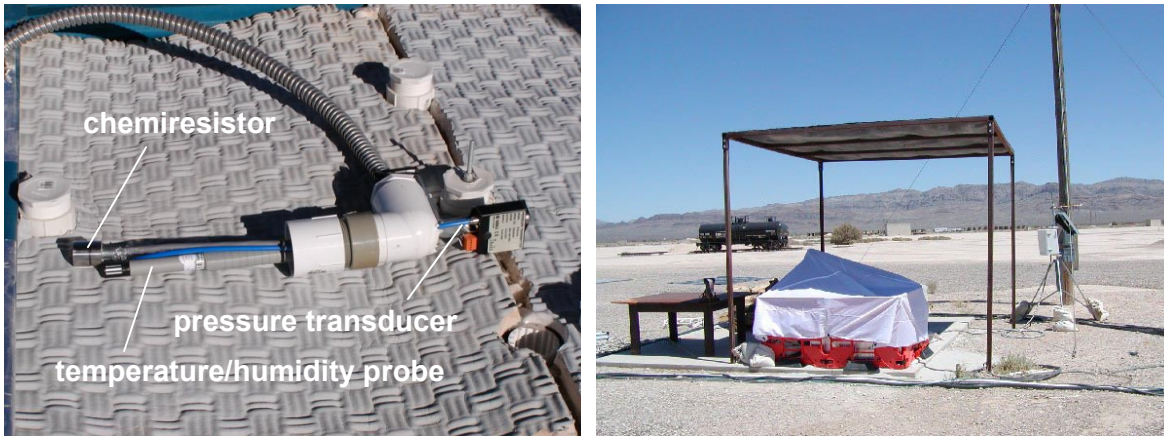
Figure 23. Left: Sensors emplaced in the sandbox. Right: Sandbox shaded from sun.
