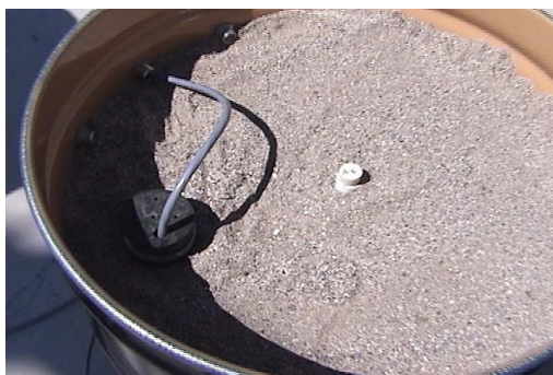
Figure 17. Top view of 55-gallon drum filled with sand. The contaminant reservoir is in the middle of the drum, and the sensor well (with sensor cable) is towards the outside.
