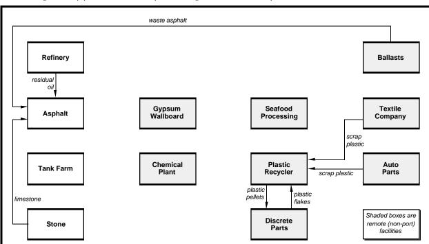
**Figure 3-3. Scenario 3: Industrial Symbiosis**The exchange of scrap plastic and waste asphalt among noncollocated companies characterizes this scenario.
