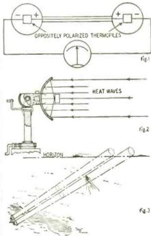
The presence of a body is indicated in one of two ways: either through direct radiation from the body, such as a smokestack of a ship (See Fig. 3.) or through absorption of temperatures when the reflector is aimed at sky, landscape or sea.
