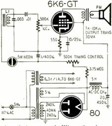
ohm timing control. When the charge on the condenser equals the ignition voltage of the neon bulb, the bulb ignites and discharges the condenser. The charging cycle begins again and will continue indefinitely. The charging and discharging surges will react on the grid circuit of the 6K6 to produce audible pulses with a tone determined by the inductance of choke and the capacity of the shunting condenser.
