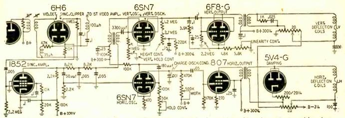
Fig. 2—Complete electromagnetic deflection system. This is better adapted to larger tubes and is used in most commercial receivers.
