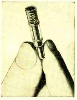
The new photocell has a diameter of 1/4 inch.
