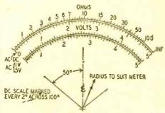
Fig. 5-Drafting details on the meter scale.
