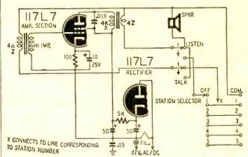
Fig. 4—A simple system which uses I tube at each end of the circuit.
