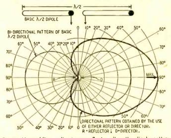
Fig. I—How adding a director or reflector alters the dipole pattern.
