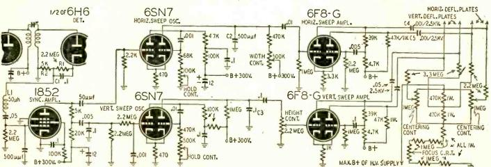
Fig. I—A typical system for electrostatic deflection of the cathode ray. This method is employed in many small television receivers.
