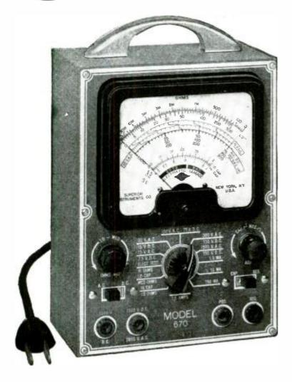
The Model 670 comes housed in arugged, crackle-finished steel cabinet complete with test leads and operating instructions. Size 5½" x 7½" x 3".
