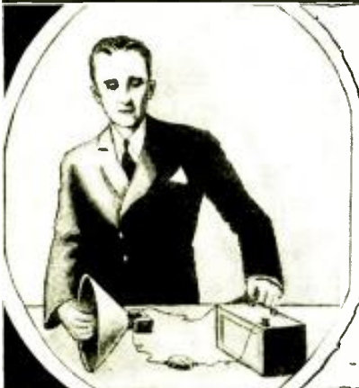
Auxiliary field coils of various resistances help the Service Man make speaker tests.
