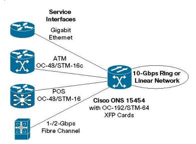
The Cisco ONS 15454 also supports lower-speed service interfaces as well, starting at 1.5 Mbps/2.0 Mbps (DS-1/E1), Ethernet, Fast Ethernet, and others to offer a complete multiservice transport solution.
